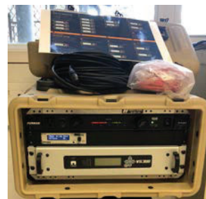
Above: A 300-watt portable emergency transmitter being tested at WCVE-FM, Richmond, VA.
